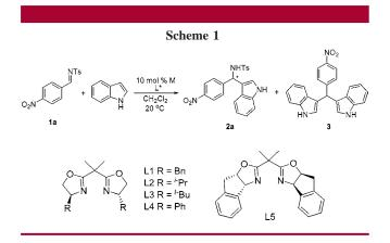
in situ by mixing  $Cu(OTf)_2$  with **L1** in  $CH_2Cl_2$  at room temperature. After adding aldimine **1a** and indole, the mixture was stirred at room temperature for 3 days. The addition product *N*-(indol-3-yl-4-nitrophenylmethyl)-4-methylbenzenesulfonamide (**2a**) was isolated in 58% yield with
